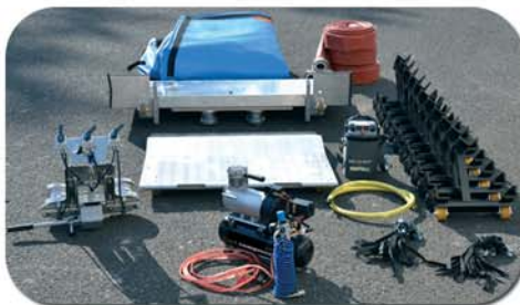
Flex-Moshon Towing System components
