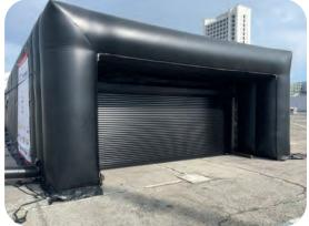
The tunnel is high enough to fit street lights and other roadside furniture for realistic test scenarios in complete darkness. The tunnel is easy to set up and can be deflated to fit into custom carrier cases.
