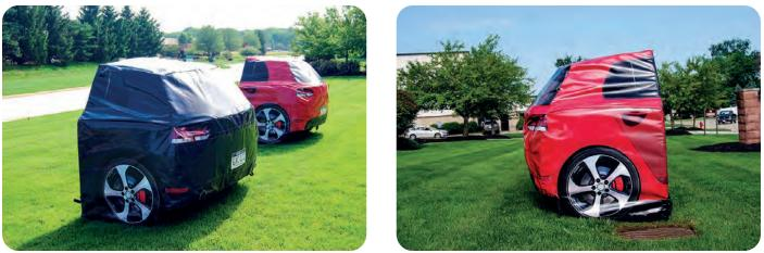
The MD-VT F is a lower cost, foam version of the official Euro NCAP Vehicle Target (EVT). It is designed to the same specifications as the Euro NCAP target and intended for development work. Being a cheaper substitute for the EVT means vehicle manufacturers and test facilities can purchase multiple vehicle targets and increase the number of tests.
