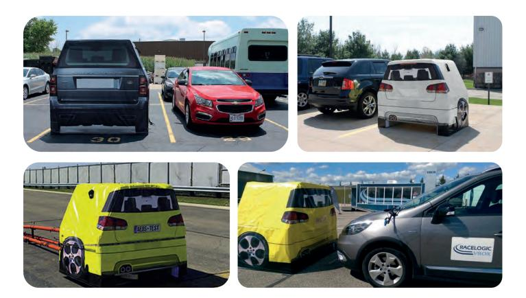
The MD-VT and MD-VT L (Large) is an inflatable, lower cost version of the official Euro NCAP Vehicle Target (EVT). It is designed to the same specifications as the Euro NCAP target and intended for development work. Being a cheaper substitute for the EVT means vehicle manufacturers and test facilities can purchase multiple vehicle targets and increase the number of tests.
