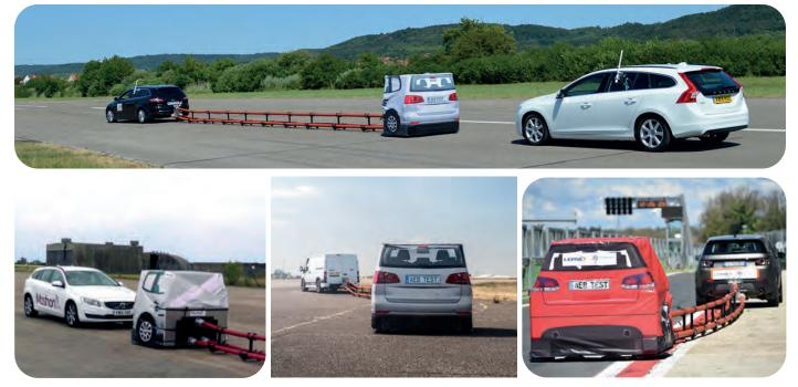
The Flex-Moshon towing system is designed to tow a balloon car during Autonomous Emergency Brake (AEB), Forward collision warning (FCW) and other ADAS tests.
