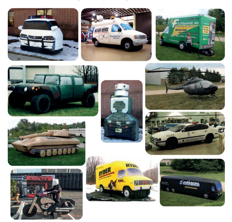
Moshon Data offers a large range of vehicle targets for ADAS testing. We also supply custom targets such as pedestrians, motorcycles, shopping trolleys and animals commonly involved in vehicle-wildlife collisions such as deer or moose. These targets can be manufactured to your individual specifications.
