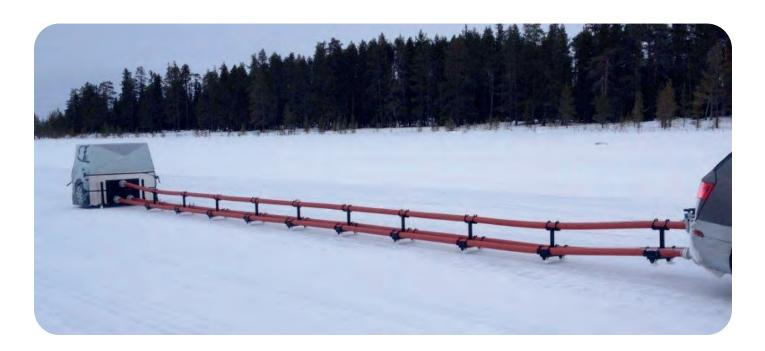
Moshon Data has developed the first Flex-Moshon EVT towing system for winter testing in the snow. Specifically adapted for winter AEB testing, the Flex-Moshon uses expertly designed skids instead of wheels which allows the towing system to glide across snow and ice.
