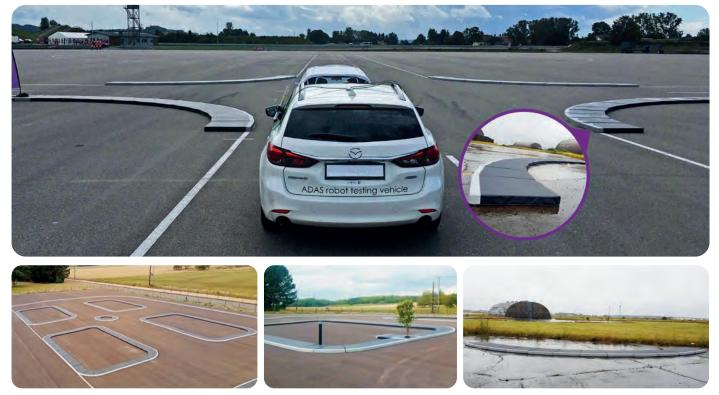
Moshon Data has designed and developed foam pavements / sidewalks in straight and curved sections to create configurable junction scenarios including Euro NCAP Car to Pedestrian Turning Adult.
