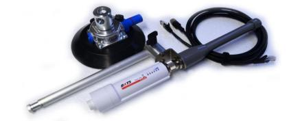
The RT-XLAN is a long range radio that extends and improves the data integrity and communication between vehicles in an RT-Range application. The RT-Range can measure the range from one vehicle to other vehicles in real-time and output its measurements on the CAN bus. It is used for the development and validation of advanced driver assistance systems (ADAS).
